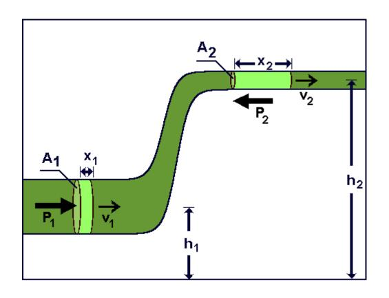
$$p_1 + \rho g h_1 + \frac{\rho v_1^2}{2} = p_2 + \rho g h_2 + \frac{\rho v_2^2}{2}$$
