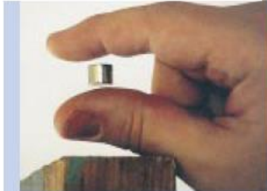
Figure 2 Levitation at your fingertips. A strong NdFeB magnet (1.4 tesla) levitates 2.5 metres below a powerful superconducting magnet. The field at the levitation point is about 500 Gauss.
